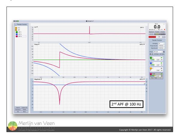
Figure 6 shows a broadband TF of a 2<sup>nd</sup> APF at 100 Hz.
